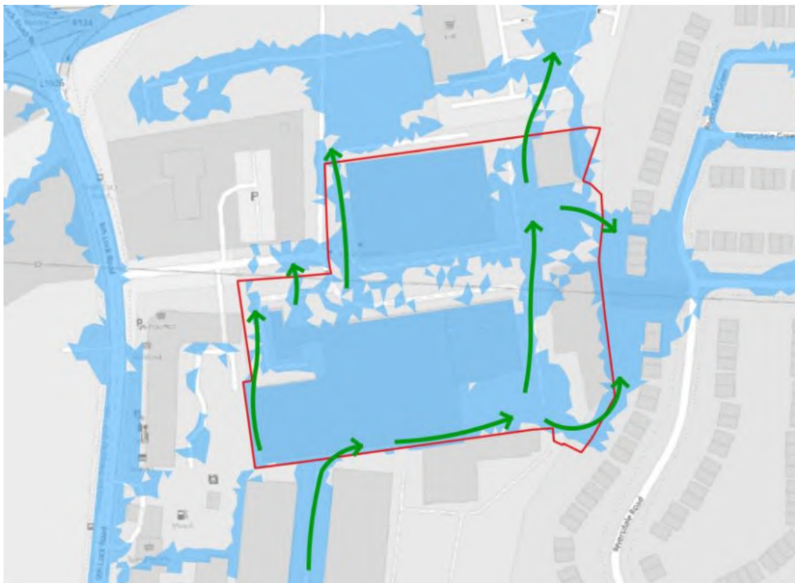
Figure 4.3: Existing Flow Route Analysis
